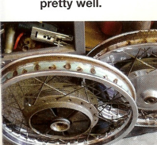
The big surprise, wheel rims rotted on the inside.
