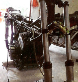
Rebuilt and re-finished forks installed.
