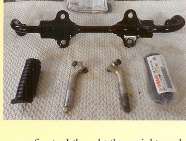
Foot pegs and mount ready to go together.
