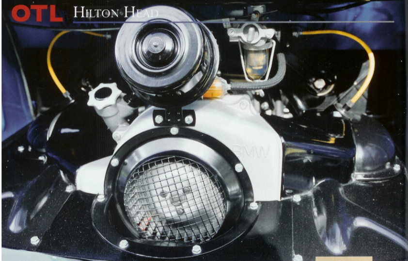
1958 "600" twin cylinder BMW air-cooled Boxer engine, installed in an Isotta built car.
