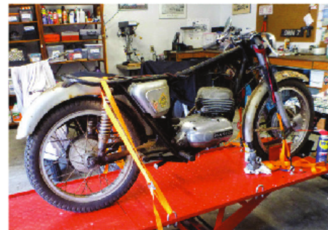
The teardown began shortly after the bike arrived. The Bultaco's 200-cc two-stroke wasn't running at the time, but the odometer showed just over 5,000 kilometers (about 3,100 miles), so chances were good that it wasn't totally worn out.
