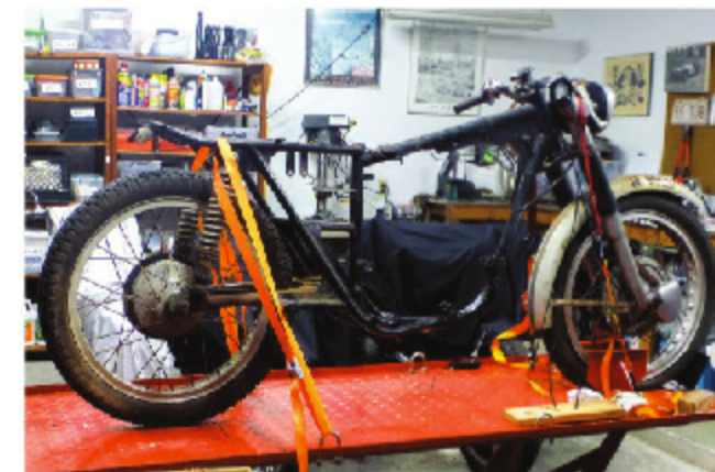
Here, with the engine out of the chassis, and the tank, side cover, and rear fender removed, the simplicity of the Metralla's frame is even more evident. Basic stuff: steel tubing, with sheetmetal gussets welded in, but still a strong and rigid foundation.
