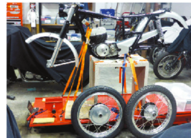
The Bul is starting to take shape with the rebuilt engine back in the refinished frame, the reconditioned forks and shocks in place, and the fenders, as well as the chain guard, bolted on. New wheels were laced up and shod with fresh rubber.
