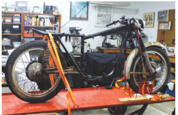
Here, with the engine out of the chassis, and the tank, side cover, and rear fender removed, the simplicity of the Metralla's frame is even more evident. Basic stuff: steel tubing, with sheetmetal gussets welded in, but still a strong and rigid foundation.
