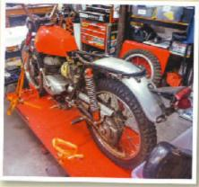
Wheels are 18-inch each plus one in width over the original. Suspension has been upgraded as well. Paint is a Toyota colour, 'Radiant Green Mica', with pearl added; the frame is gloss charcoal. All-up weight without fuel is 198lb. The motor is probably making 35bhp or more. It goes quite nicely and I'm very happy with the result. There is more information on my website. Hope you like it.
